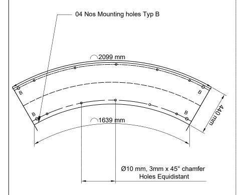
Plate- Mild Steel Chequred Sheet 10 mm Thickness Side Strip - Mild Steel (20 mm X 20 mm)
