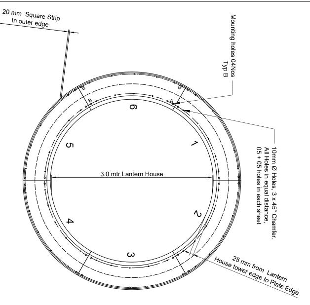
\* Out side gallery is made up of 06 Nos of Chequred Sheets out of which 02 Nos are to be replaced.
