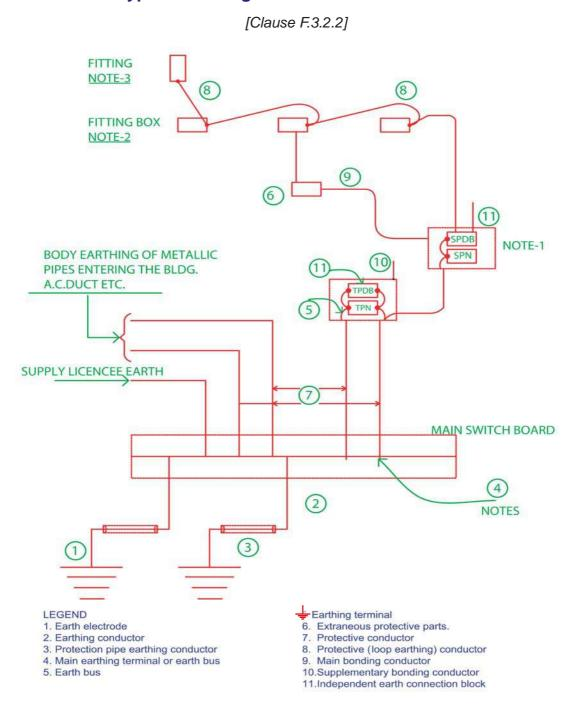
NOTE 1. (8) Should be terminated to (11) by screws.
