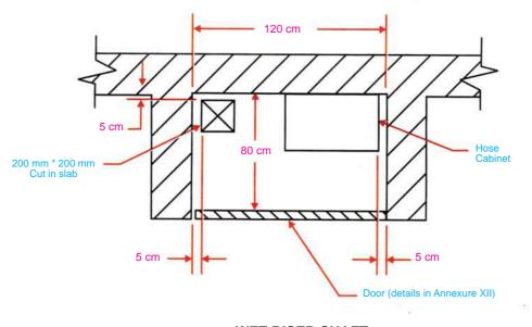
WET RISER SHAFT one for 1000 sq.mtrs Floor Area
