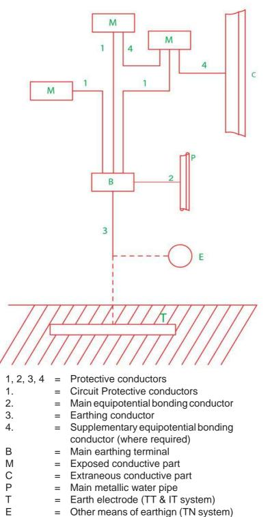
Typical Earthing Schematic For Internal E.I.
